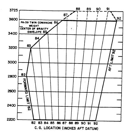
Moment change due to retracting Landing Gear = +1266 in.-lbs.
